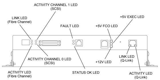
Figure 6-1 Bottom View of the Type C Fibre Channel Bridge/Router (FCO)
